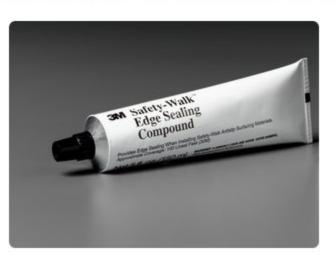
3M™ Safety-Walk Edge Sealing Compound is a liquid, solventbased sealer that protects exposed edges of slip-resistant tapes and treads from excessive moisture or liquids. One 5-ounce tube with convenient tube applicator seals approximately 75 to 100 linear feet.
